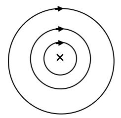
**Current direction** Concentric circles Magnetic field direction
